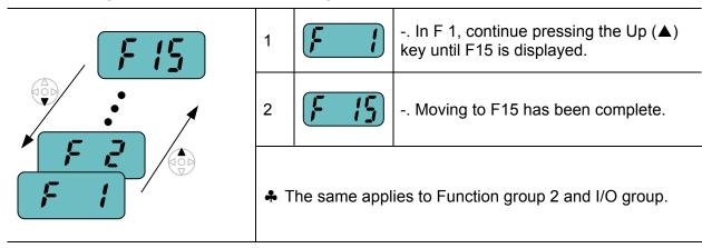
♣ Note: Some codes will be skipped in the middle of increment (▲)/decrement (▼) for code change. That is because it is programmed that some codes are intentionally left blank for future use or the codes user does not use are invisible.
