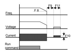
In case of DC brake at high load inertia and frequency, change the DC brake controller gain according to H37 set value.
